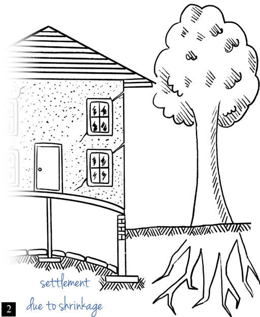
2. Tree roots can dry out the soil and cause differential settlement to building
